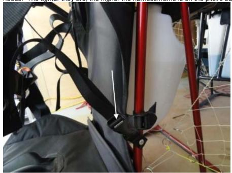
g. There are two chest straps. The main chest strap (the lower of the two) must be tightened just enough to keep the suspension bars from separating around the circular contact point with the frame. In other words, there should be no space
