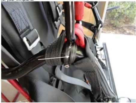
c. Adjust the leg straps so that they are comfortable. The leg straps have no other function other than for safety and comfort. If they are too loose, the pilot may have difficulty sitting in the harness after launch. They are too tight, he may trouble running in the harness. When the pilot stands up in the harness, there are other straps that keep the harness from getting to low on the pilot.
