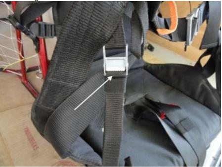
f. The last adjustment must be done while the pilot is standing up. Tighten the straps indicated in the photo below to make the harness/frame high enough so that the pilot can comfortably run while launching. If the shoulder straps are too loose, there will be problems getting this adjustment correct. These can be as tight as the pilot needs. The tighter they are, the higher the harness/frame is on the pilot's back.
