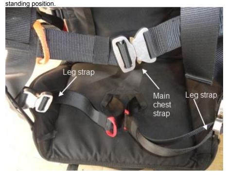
h. Finally, sit in the harness again and check all adjustments. Some of these adjustments, such as the seat angle, can be made while flying when safely away from the ground.
