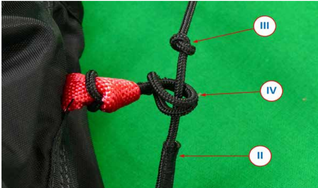
Photo K: Pass II through the larks head knot on IV, above the adjustment knot III.
