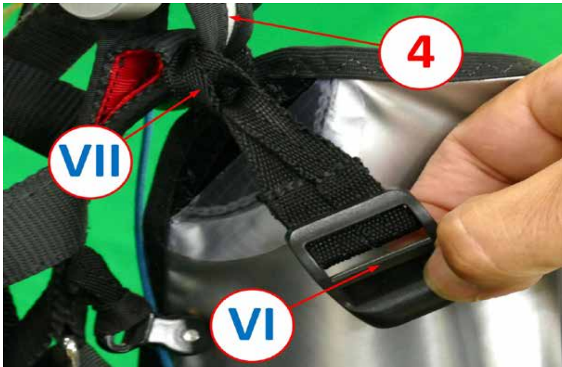
Photo Q: Then, pass VI (the ladder-lock slider) through its own webbing loop, and tighten the knot against the harness.
